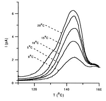
Fig. 5. Effect of the polarization window width on the TSDC discharge of PMMA electrets formed by WP. Polarization parameters:  $T_p = 135^{\circ}$ C,  $V_p = 1000$  V,  $t_p = 40$  min,  $T_0 = 110^{\circ}$ C,  $t_s = 5$  min,  $\beta = 2.5^{\circ}$ C/min, window width  $\Delta T_w$  as indicated in the figure.
