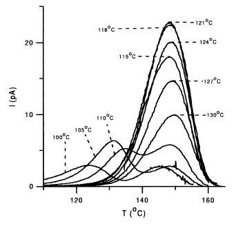
Fig. 3. TSDC discharges of windowing polarized PMMA electrets. Polarization parameters:  $T_p$  as indicated in the figure,  $V_p = 5000$  V,  $t_p = 15$  min,  $T_0 = 80^{\circ}$ C,  $t_s = 2$  min,  $\beta = 5^{\circ}$ C/min, window width  $\Delta T_w = 0$ .
