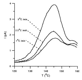
Fig. 6. Effect of the cooling rate on the TSDC discharge of PMMA electrets formed by WP. Polarization parameters:  $T_p = 135^{\circ}$ C,  $V_p = 1000$  V,  $t_p = 40$  min,  $T_0 = 110^{\circ}$ C,  $t_s = 5$  min,  $\Delta T_w = 0$ , heating rate  $\beta = 2.5^{\circ}$ C/min, cooling rate as indicated in the figure.
