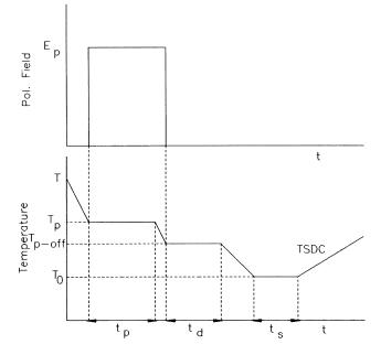
Fig. 1. Thermic and electric treatments to form electrets by windowing polarization.
