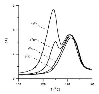
Fig. 4. Effect of the polarization window width on the TSDC discharge of PMMA electrets formed by WP. Polarization parameters:  $T_p = 125^{\circ}$ C,  $V_p = 1000 \text{ V}$ ,  $t_p = 40 \text{ min}$ ,  $T_0 = 100^{\circ}$ C,  $t_s = 5 \text{ min}$ ,  $\beta = 2.5^{\circ}$ C/min, window width  $\Delta T_w$  as indicated in the figure.
