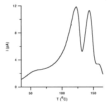
Fig. 2. TSDC discharge of a conventionally polarized PMMA electret. Polarization parameters:  $T_p = 135^{\circ}$ C,  $V_p = 500$  V,  $t_p = 45$  min,  $T_0 = 30^{\circ}$ C,  $t_s = 5$  min.
